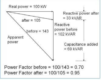
Figure 4. Effect of Power Factor Correction
