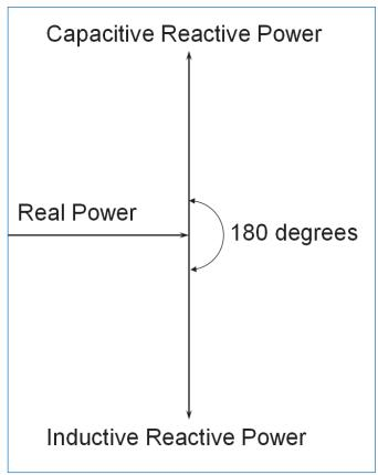
Figure 3. Capacitive Reactance/Inductive Reactance
