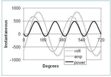
Figure 2. 0.7 Power Factor at 200kW
